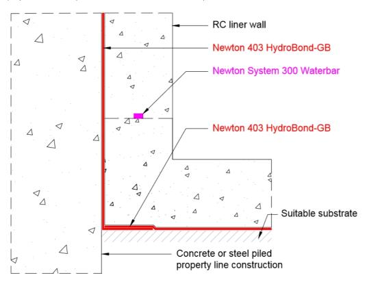
Figure 2 - typical movement joint
