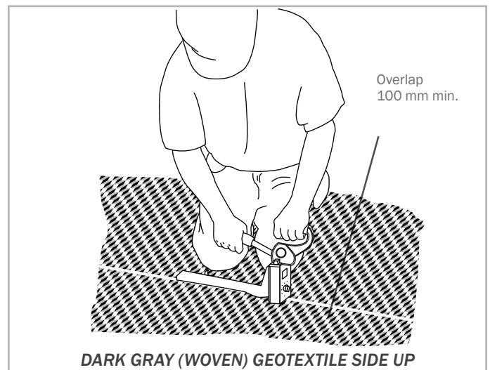
Figure 1.2 – Secure overlaps together with fasteners
